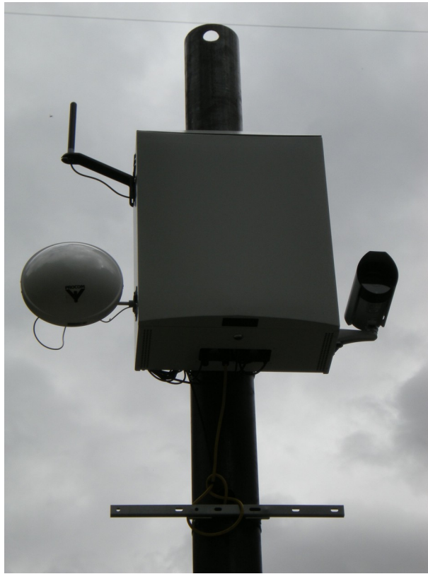
Figure 5: System for mudslide and debris flow with Radar-antenna, UMTS-antenna, housing and IP-camera
