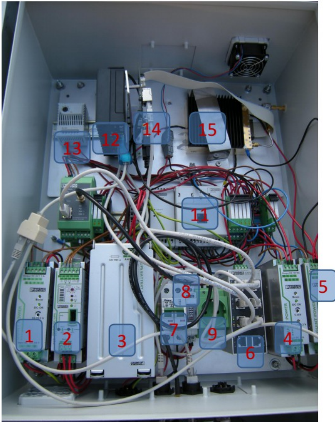
Figure 6: Electrical supply components of the Radar and the Radar module (15)
